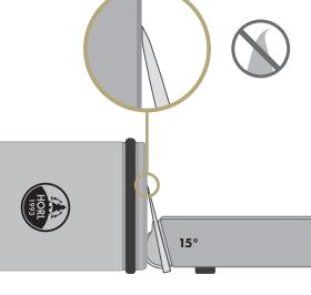
Before using the corundum whetstones, make sure that your knife is ground in on both sides with the HORL® Standard Diamond. The cutting edge should be burr free to prevent massive abrasion of the stones.
