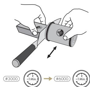
Use the sharpener and the angle support as usual. For the best finish, refine both sides of the blade for the same amount of time.
