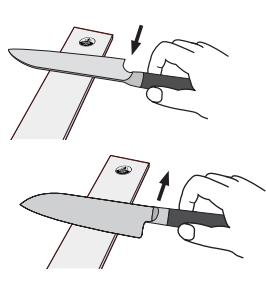
The HORL leather removes even the finest grinding residue. Just wipe the blade over it alternately with both sides of the knife as you were buttering bread.
