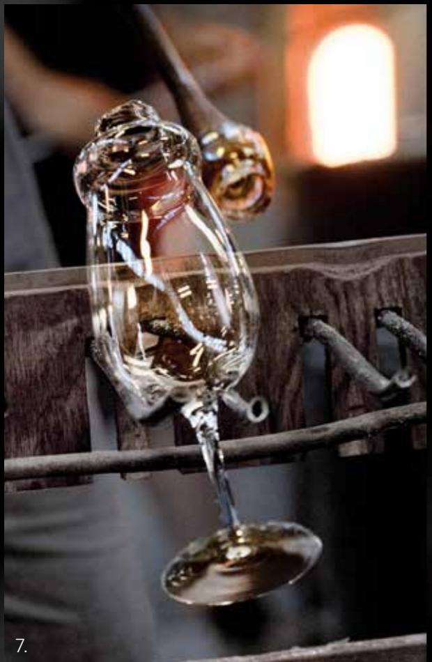
7. The assistant knocks the glass off the blowpipe using a special holder known as a carry-in-fork. The glass is then fetched by a carrier, who places it in a lehr, where it is slowly cooled. After cooling, an initial quality assurance check is carried out by a sorter. If the glass is deemed to comply with Orrefors' stringent quality standards, it is sent for further processing.
